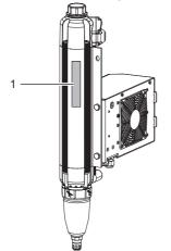
1 Membrane drying unit type plate
