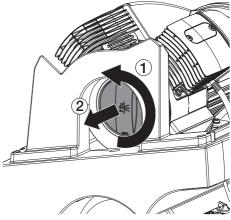
> Remove the air intake filter.
