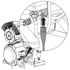
Secure the mains connector using the cable tie provided.
