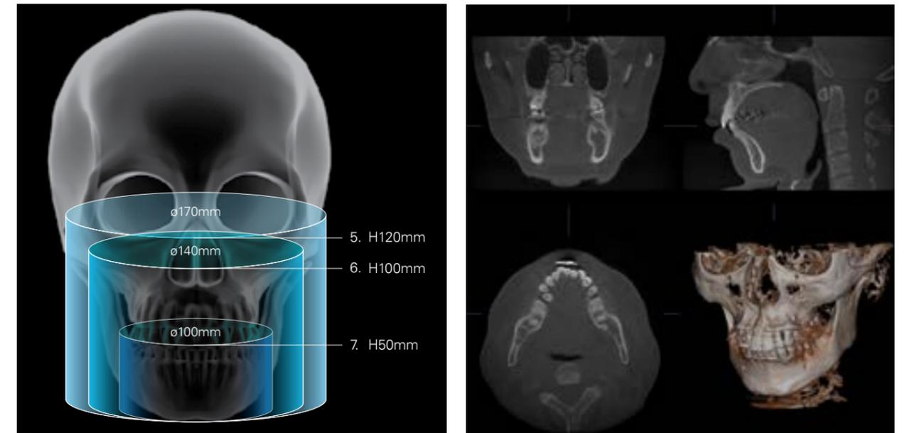
4.  $\phi 170 \times H 120$  mm (250 $\mu\text{m}$ )
